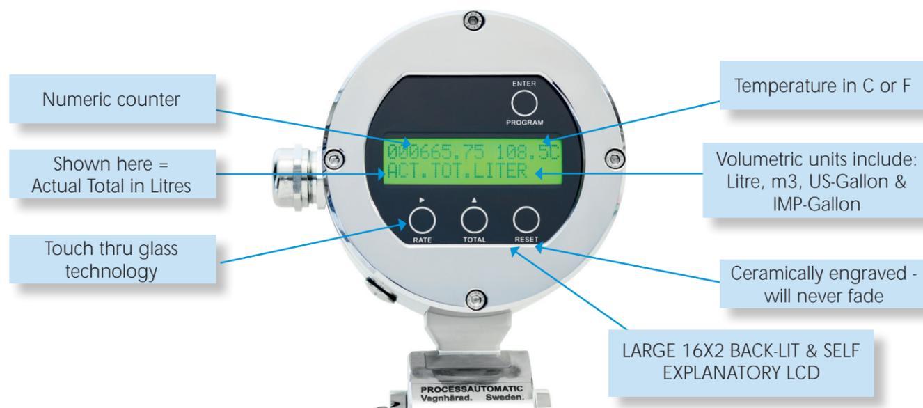
The EZ-2US Flow Computer has a large 16 x 2 back-lit LCD that shows Rate, Resettable Total and Resettable Accumulated Total. If opted, the fluid temperature is also clearly visible on the LCD with temperature unit. The EZ-2US allows for full programming of EZ-Mag, with an easy to use and self explanatory touch thru glass display.
