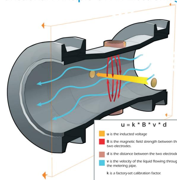
When a conductive liquid flows through the magnetic field, a voltage is induced. This voltage is proportional to the velocity of the flow and is accurately measured by two electrodes. The electrodes are mounted opposite each other on the inside of the metering tube.
